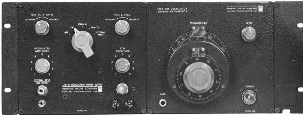
Figure 1-2. The VHF Oscillator and the 1264 Modulating Power Supply assembled with the Type 0481-P416 Adaptor Plate Set for rack mounting.
