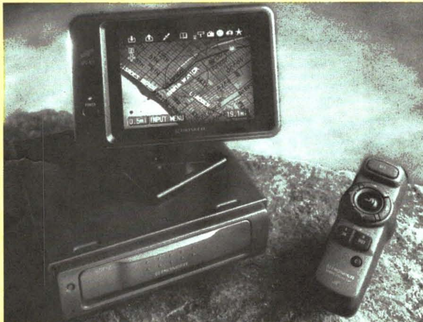
Pioneer's GPS-X77 uses a proprietary map database. The vehicle location is indicated on the moving-map display, and a synthesized voice calls out route-guidance instructions.
