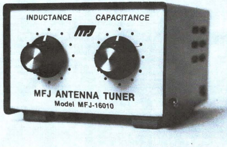
The go-anywhere MFJ-16010 Randomwire Antenna Tuner is small enough to carry in your pocket or briefcase and covers all bands from 1.8 to 30 MHz continuously.
