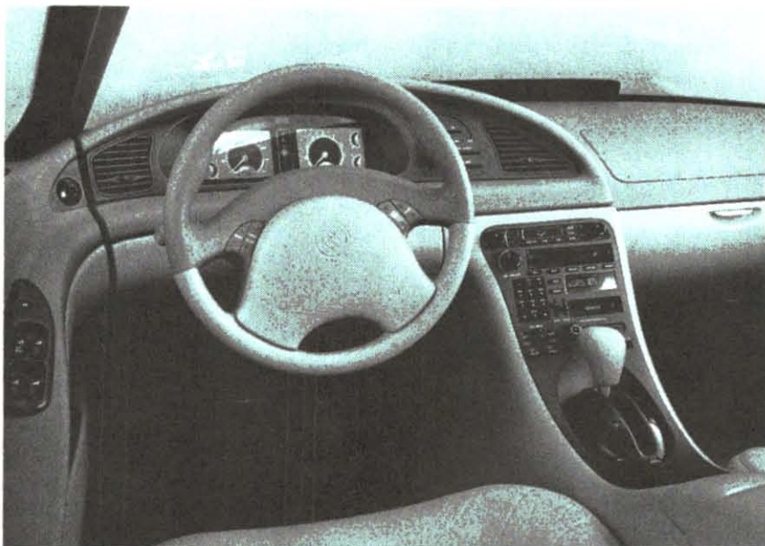
The XP2000's full-color, flat-panel display is configured here to present the normal information on speed, engine rpm, and status of the engine. Information from the Smart Arrow Navigation System is shown on the heads-up display just above the top of the steering wheel
