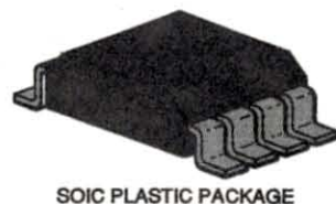
Fig. 3. The SOIC gull-wing, plastic integrated-circuit package is so tiny, the leads have only a 0.050-inch space between them.
