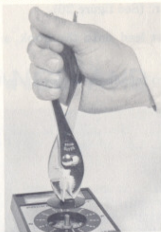
Fig. 21 Removal of Permutator Switch Knob for Disassembly
