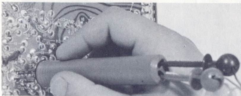
Fig. 8 Using 39G85 Touch Test Probe
