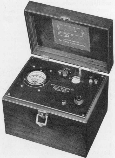
TYPE 532 Station Frequency Meter
