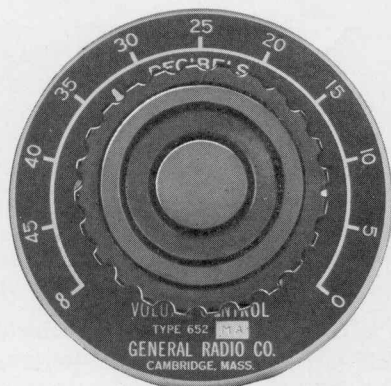
FIGURE 6. A dial from a TYPE 652 Volume Control
